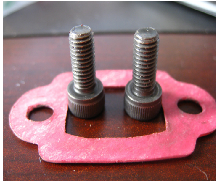
Original gasket and bolts (5mm x 12mm)
