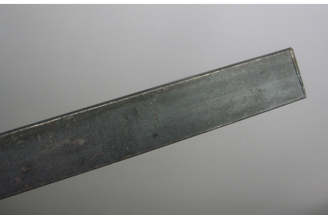
Steel bar - 3/4" wide x 1/8" thick x whatever length the store sells it at
