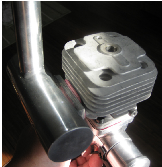
Typical way of attaching a side muffler to engine
